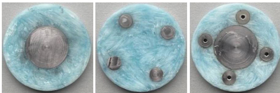
Fig. 4: GFRP with bonded-in steel drill bushings.
