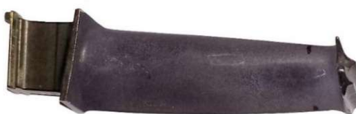
Fig. 2: The turbine blade after the service life
