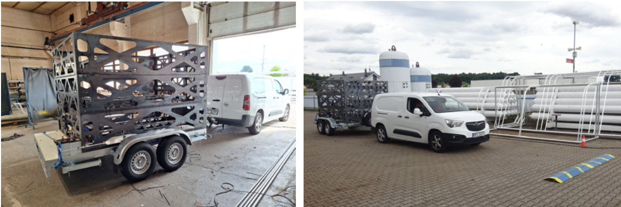
Fig. 3: Trailer attached to an Opel Combo and passing over an artificial vertical bump.
