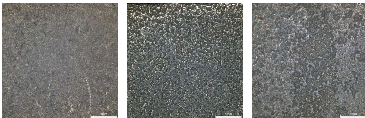
Fig. 3: The turbine blade coating damage during the service life: initial (after GO procedure including ground test: less than 1% coating damage - left), first visual detectable damage (after 520 Flight hours: 13% coating damage - middle), major damage (after 819 Flight hours: 32% coating damage - right)
